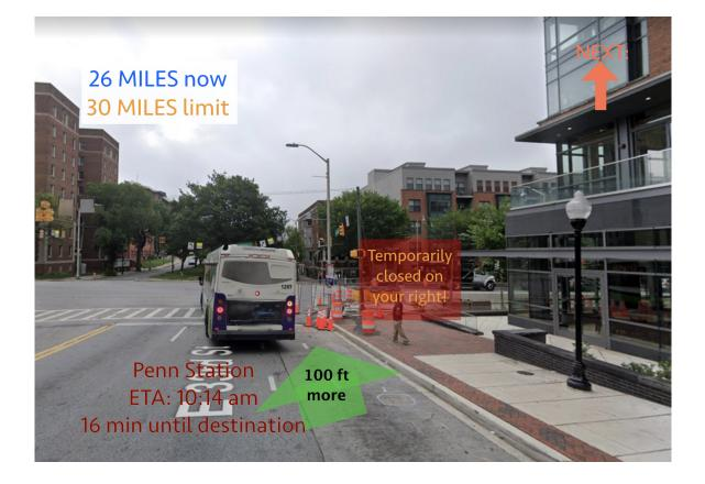
Prototype #2 demonstrates how the google glass navigation guide can display real-time road conditions. The device notifies the user that the street on the right is temporarily closed due to construction, so that the user knows to avoid it. The device will calculate the optimal route, taking into account traffic and road conditions.
